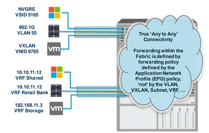
• Forwarding is fully decoupled, flattened IP address space
