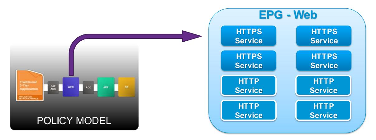
**EPG**s are a **grouping of end-points** representing **application or application components independent** of other network constructs.
